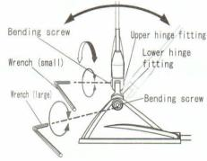
To remove the antenna element When washing your car, the antenna element can be taken off. Please remove the antenna element by hands.
