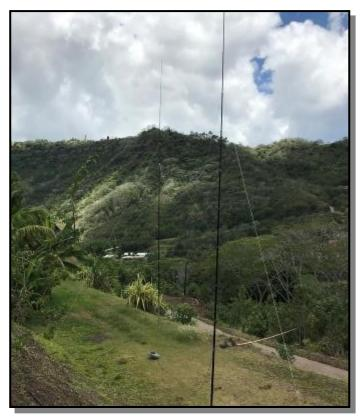
One Hexbeam was used primarily for 12 and 20 meters and placed directly behind the pension.
