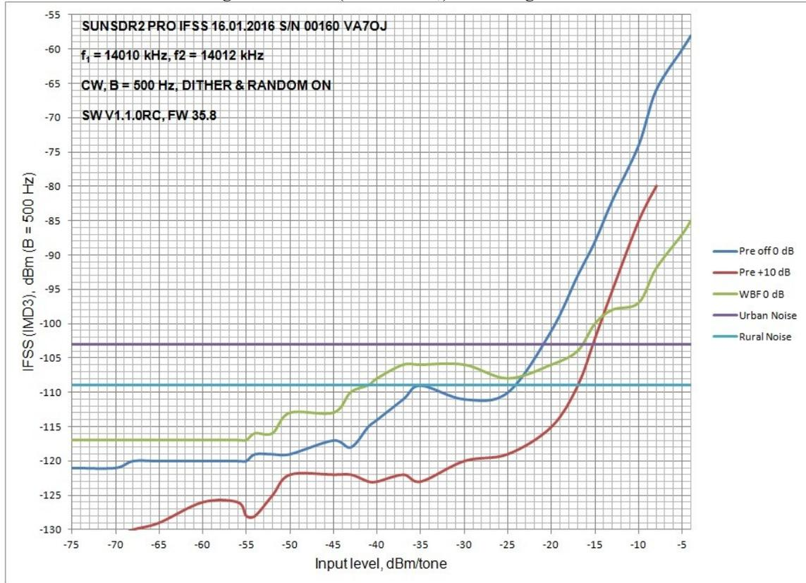
It will be seen from Figure 5 that the  $IMD$  product amplitude crosses the typical urban band noise line for per-tone input levels  $< -21$  dBm with Preamp off and  $< -15$  dBm with +10dB Preamp on. This is now comparable to other direct-sampling SDR's I have tested. The 'Preamp off' curve is now below the rural band noise line for input levels below -24 dBm/ton, except for one point at -35 dBm/ton. This is a very significant improvement over the IFSS test results of 28.8.2015. (See page 5).
