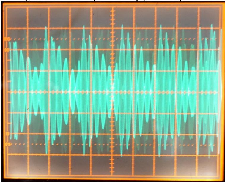
**15. ALC Compression Check.** In this test, a 2-tone test signal is applied to the MIC jack from an audio generator. An oscilloscope is connected to ANT3 via a 45 dB high-power attenuator.
