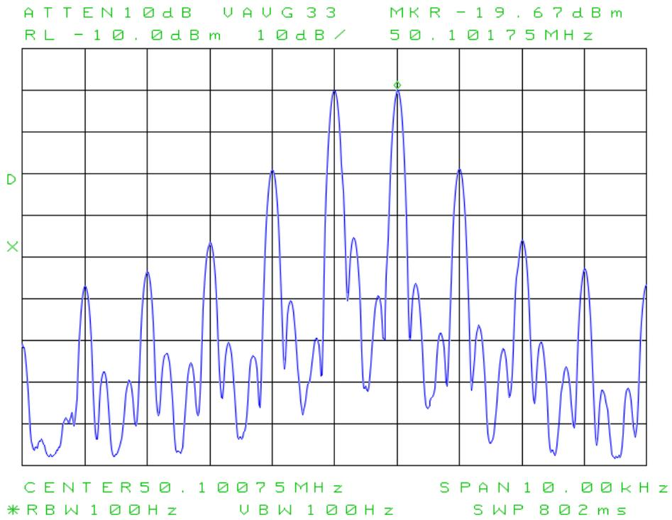
**Figure 13: Spectral display of 2-tone IMD at 144.1 MHz, 6.3W PEP.**
