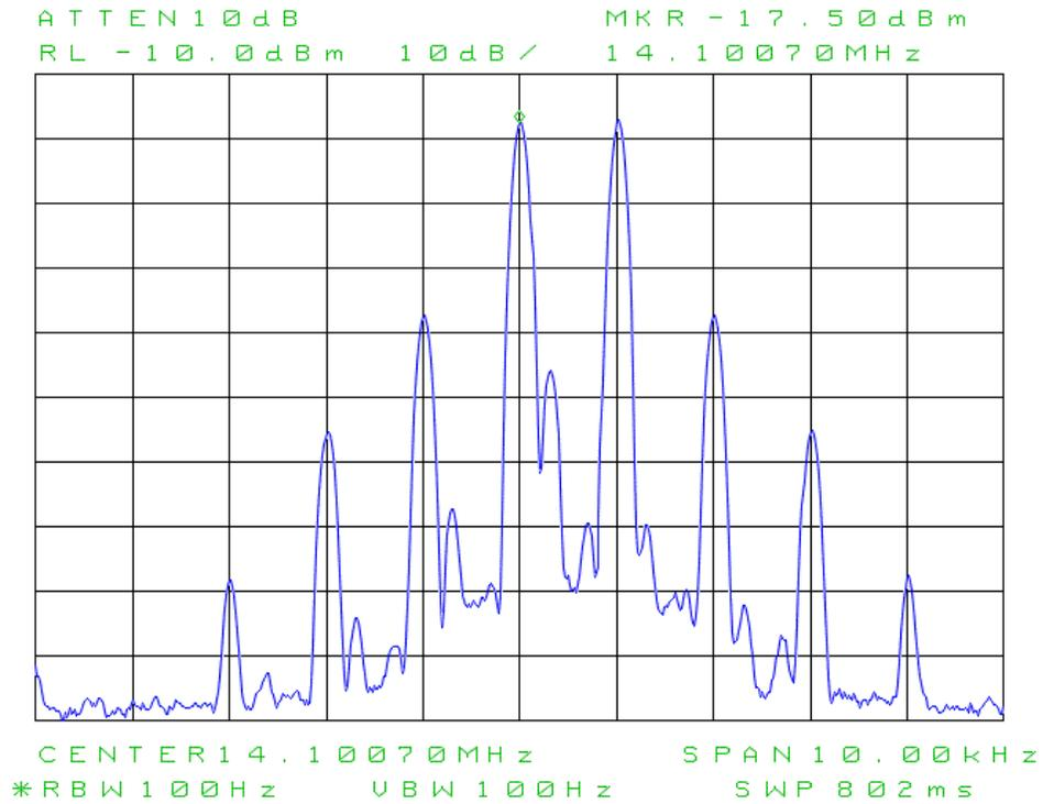
**Figure 26: Spectral display of 2-tone IMD at 50.1 MHz, 14W PEP.**
