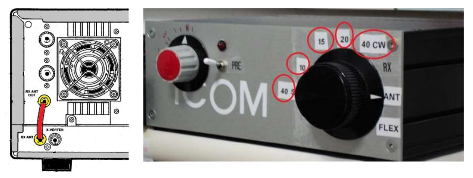
If your RX has a poor out of band rejection (Rate C-D), I would first place an external narrow BPF, as per the one above, actually even if it does have a fairly good out of band rejection (rate B). Is any thing missing?
